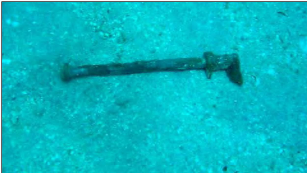
Figure 25. Copper or bronze alloy drift pin, which was a common characteristic of nineteenth-century ship construction (courtesy of Charles Consolvo).
