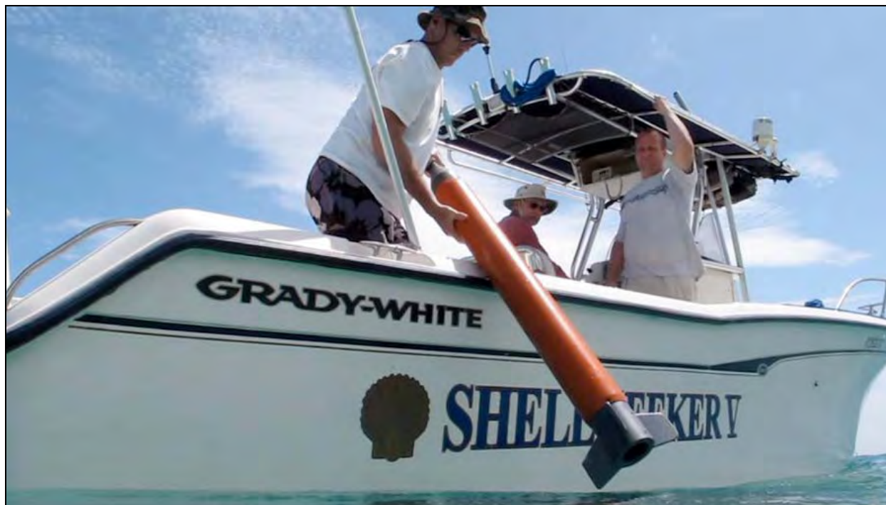
Figure 37. The Shell Seeker V , a 26-foot center-console, Grady-White employed for both survey and diving. Mr. Charles Consolvo, Director of the Trust, Project Manager of the investigation, and vessel owner is at the helm. Pictured is the magnetometer being deployed (courtesy of Erik Miles).
